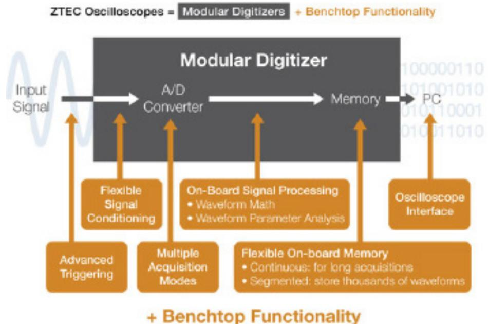
Figure 2: Modular Oscilloscope Features
