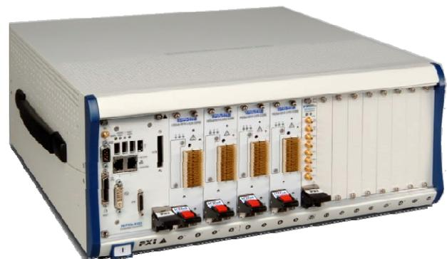
Figure 1: High Speed Subsystem device. To the left end of the chassis is the embedded controller, in the slots are Teradyne LVDS core instruments.
